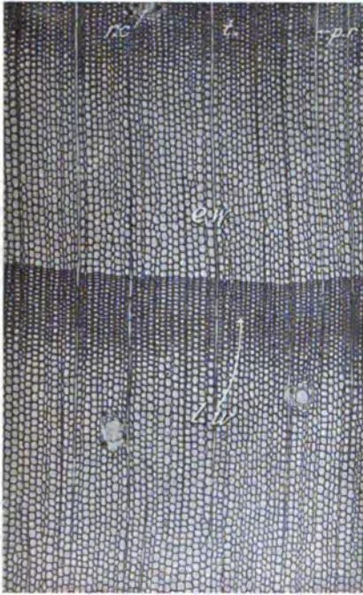
FIG. 331.—Transverse Section of Norway Pine. Magnified 25 Diameters. (Bull. 139, U. S. For. Ser.)
